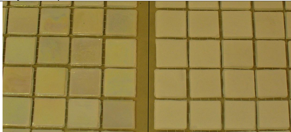
a) Mosaico 1 / SAMPLE MOSAIC 1 with TiO_2 | b) Bianco 1 / SAMPLE 1 without treatment
